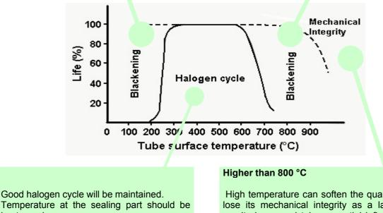
Temperature at the sealing part should be kept much prevent premature failure.
