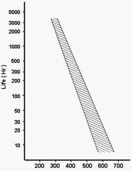
Temperature at sealing part (°C)
